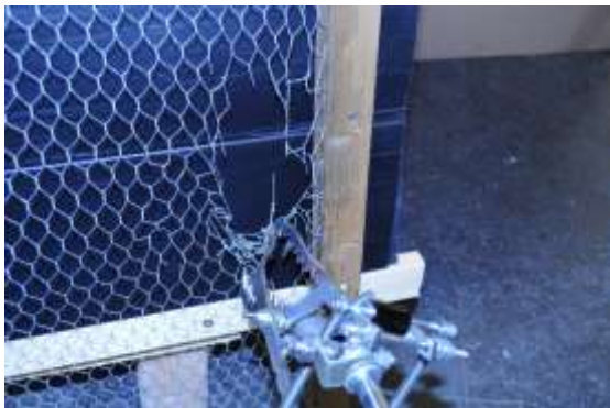
Figure 17: Chicken wire is particularly weak when subjected to simulated fox attacks, lasting mere seconds
