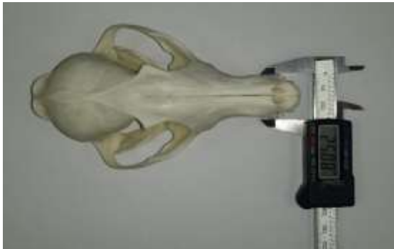
Figure 40: Framework and mesh apertures of 25mm and larger will allow a fox's jaw to apply full force while attacking
