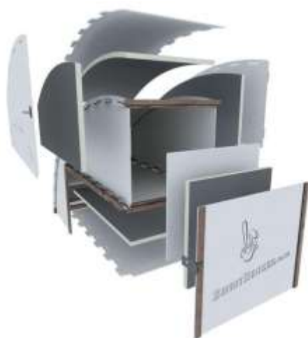
Figure 6: An exploded view of an example of a fully insulated sleeping area
