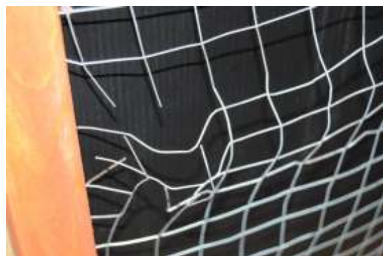
Figure 15: This 21 gauge (0.8mm) 25mm aperture galvanised weld mesh quickly failed in a matter of seconds during a simulated fox attack
