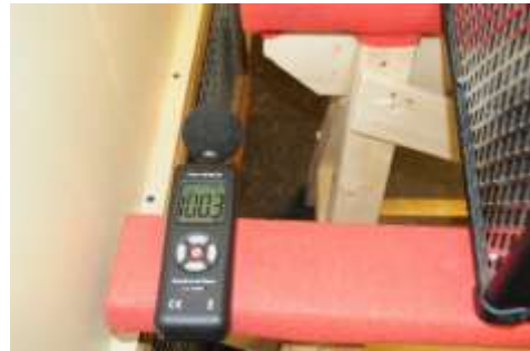
Figure 52 the amplifier set to 100dBA at the first frequency of 125Hz
