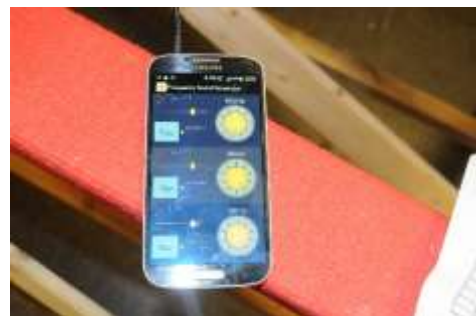
Figure 53: a smartphone is capable of being used as a tone generator for testing specific frequencies
