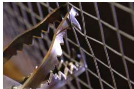
Figure 43: Gnaw test on mesh using a fox jaw facsimile
