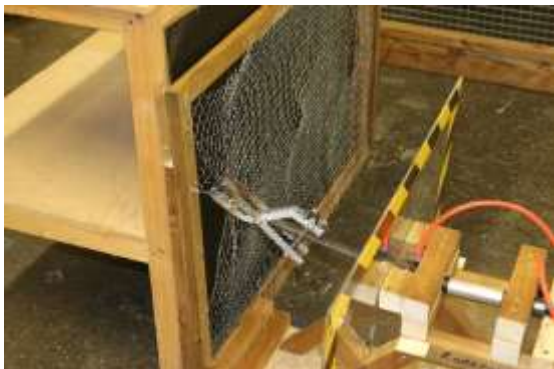
Figure 18 . Meshes fixed using only staples will also fail after only a few minutes
