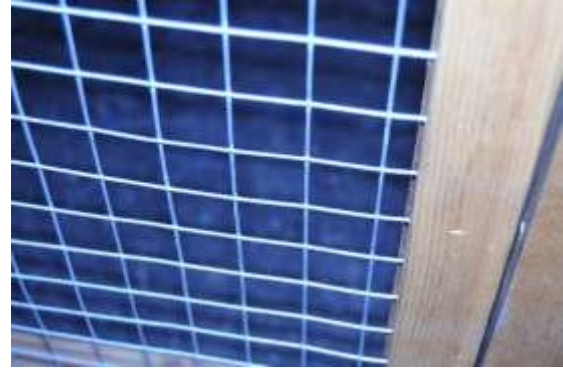
Figure 19: This 17 gauge weld mesh secured with trims is seemingly untouched after a prolonged simulated fox attack
