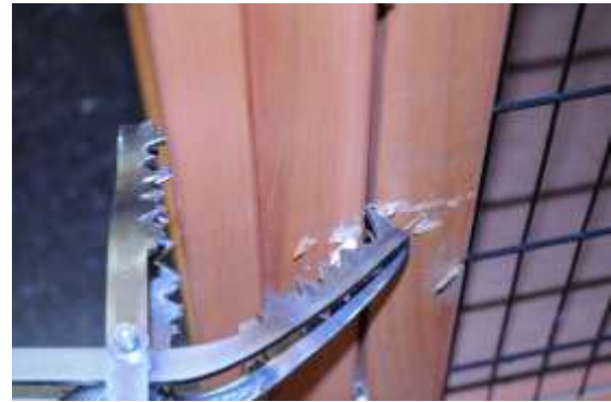
Figure 20: Some soft timbers, while resisting a simulated fox attack, are easily damaged
