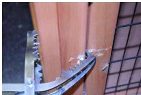
Figure 3: Rotten timber, as shown above, will weaken the structure and attached mesh leaving rabbits vulnerable to attack. (photo credit: Beentree)
