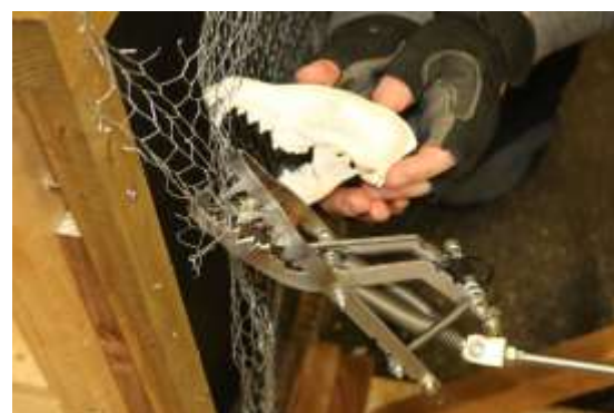
Figure 39: The results of jaw pull testing on chicken wire, real fox skull for comparison
